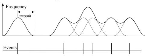
The diagram shows the result of using the built-in raised cosine waveform. The area under the curve for each spike is 1. You would normally use a smoothing period that covered several events to obtain a smooth output.
