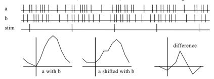
If the stimulus channel holds events at some constant interval int, by shifting all events on one of the two channels by int, the only correlation between the two channels left is the correlation due to the stimulus. Thus by forming the difference between the unshifted correlation and the shifted correlation, you can obtain the correlation between a and b with the effect of the stimulus removed.
