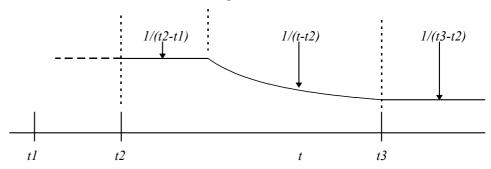
The diagram shows the result when there are three events at times t1, t2 and t3. The output from t1 to t2 depends on what happened before t1. From time t2 to t2+(t2-t1), the output is the reciprocal of the previous interval. From this point onwards to t3, the output reduces until at t3 it becomes 1/(t3-t2).
