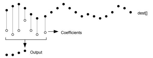
This diagram shows the general principle of the FIR filter. The hollow circles represent the filter coefficients, and the solid circles are the input and output waveforms. Each output point is generated by multiplying the waveform by the coefficients and summing the result. The coefficients are then moved one step to the right and the process repeats.
