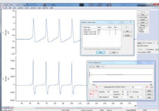
Dynamic clamp simulating action potentials with model parameter access during sampling
