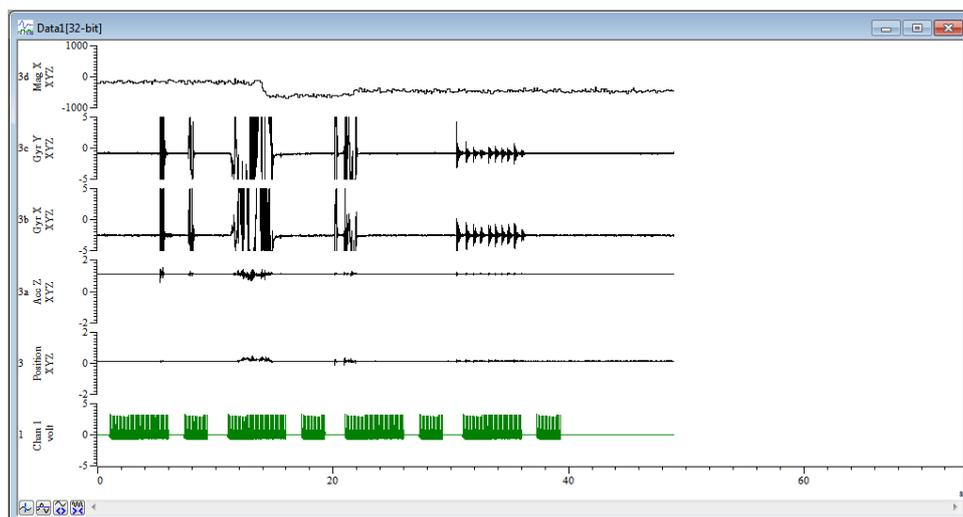
An ordinary waveform channel is shown at the bottom, above which are data from two of the three MPU9250 accelerometer axes, then two gyroscope axes and the staircase-like, slower magnetometer data. Note that the baseline level for the upper accelerometer channel is about 1, rather than 0 as in the other. This is because it is showing the Z axis which registers Earth's gravity field.
