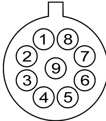
*ODU front-panel connector pinout*
