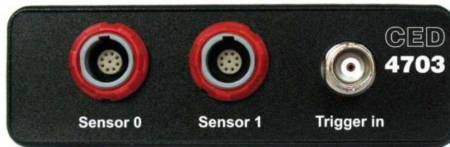
*Sensor input* The sensor inputs, Sensor 0 and Sensor 1, accept digital data, either in SPI or I<sup>2</sup>C format, from a range of sensors. The range will be added to from time to time, according to demand and as new devices become available. For information on two sensors documented in this manual, see page 20 onwards.
