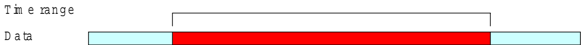
Process with non-triggered analysis. All data in the time range is included in the analysis
