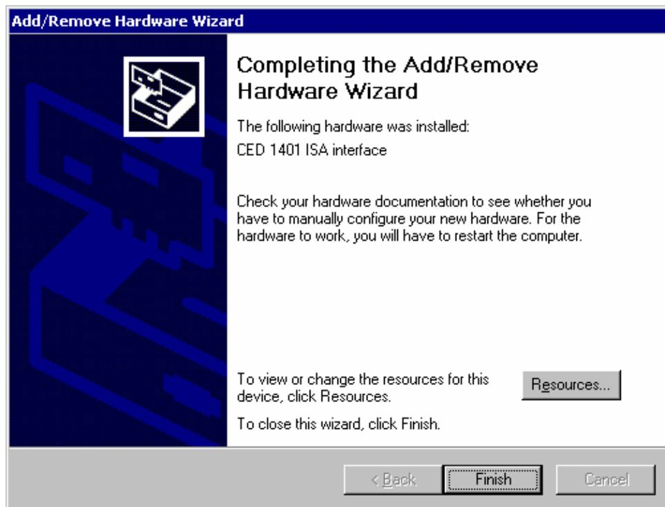
**The I/O base address** The installer sets a default I/O base address of 300. This matches the default address set by links on the interface card (see page 25 for details.) If you are using this default address, simply press *Finish* to complete the installation. If your card's address has been altered, e.g. to avoid clashes, the software I/O address must be set to the correct range before installation. Changes to interrupt and DMA channel are dealt with automatically.
