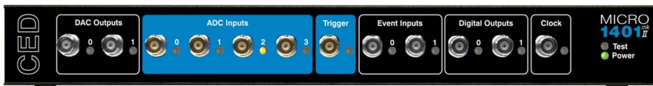
**Waveform input** Waveform input channels are buffered through unity-gain amplifiers. Channels are then steered into the ADC (Analogue to Digital Converter) via a multiplexer. The input sample-and-hold is part of the ADC chip. The ADC converts an input voltage to a 16-bit digital value in approximately 2  $\mu$ s. Optionally, a second sample-and-hold can be fitted to channel 3, which can then be sampled simultaneously with one of the other three channels.
