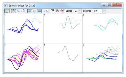
The window is linked to the Edit WaveMark dialog. Double-click a cell to open the Edit WaveMark dialog. Single-click a cell to select the corresponding channel in the Edit WaveMark dialog. The display is controlled by the toolbar at the top of the window. The toolbar commands are:
