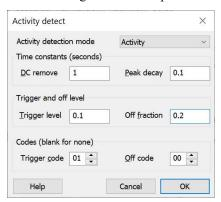
This process works on a rectified version of the input signal after DC removal. It works as a state machine with 3 states:
