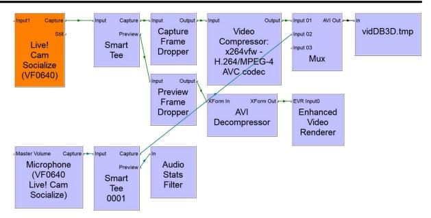
Note that this example graph (using an AVI file format and the x264 video compressor) does not match the Copy Graph output, above. The arrows show the direction of data flow between the filter *Pins* (a pin is a possible connection point of a filter). The various filters that can appear in the graph are:
