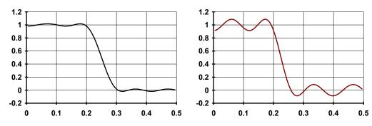
This is illustrated by these two graphs. They show the linear frequency response of two low pass filters, both designed with 18 coefficients (we have used so few coefficients so the ripple is obvious). Both have a pass band of 0 to 0.2, but the first has a gap between the pass band and the stop band of 0.1 and the second has a gap of 0.05. We have also given equal weighting to both the pass and the stop bands, so you can see that the ripple around the desired value is the same for each band.
