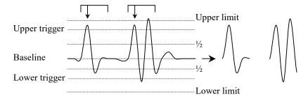
With multiple traces, each trace is tracked separately and the first trace to trigger saves the data for all traces.
