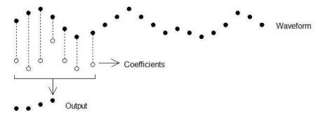
This diagram shows the general principle of the FIR filter. The hollow circles represent the filter coefficients, and the solid circles are the input and output waveforms. Each output point is generated by multiplying the waveform by the coefficients and summing the result. The coefficients are then moved one step to the right and the process repeats.
