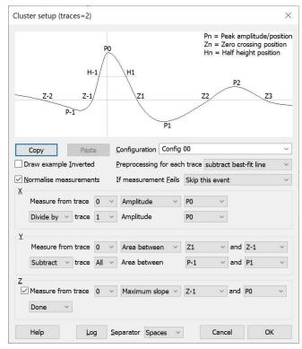
The dialog has 4 main regions: a schematic of a spike trace to use as a reference when selecting measurements, general controls, definitions of the x, y and z measurements, and the buttons to close the dialog. The dialog controls are:
