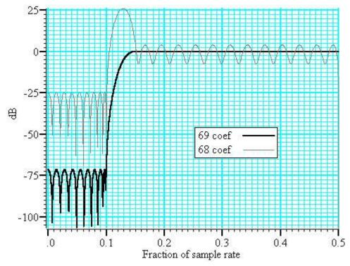
The graph shows the results of this high pass filter design with 69 coefficients, which gives a good result, and with 68 coefficients, which does not. In fact, if we had not given a factor of 10 weight (20 dB) to the stop band, the filter with 68 coefficients would not have achieved any cut in the stop band at all!
