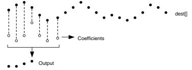
This diagram shows how the FIR filter works. Open circles represent filter coefficients, solid circles are the input and output waveforms. Each output point is generated by multiplying the waveform by the coefficients and summing the result. The coefficients are then moved one step to the right and the process repeats.
