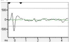
The two black triangles mark the start and end of the region of the spike that is passed to the template matching system. Click on a triangle and drag to change the region. When you drag the markers, vertical cursors drop down to identify the selected area.
