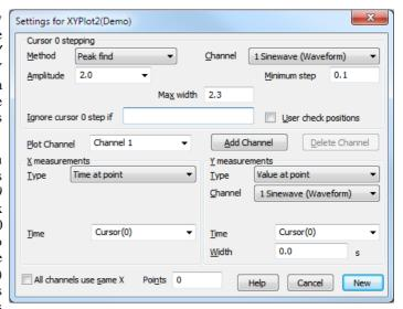
A Process command sets the data region to search for cursor 0 step points, exactly as for the result view analysis commands. You can process data both on-line and off-line. Processing can take a while if there are many cursor 0 steps to do. A progress dialog appears in a long process to allow you to stop early.
