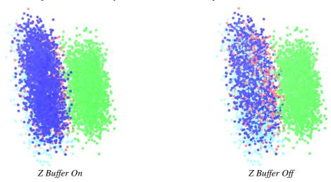
The use of the Z Buffer is recommended if you use the <u>Colour Fade with Z</u> or <u>variable dot size</u> options. You should only need to turn it off if you have a very large number of points to display and the display response has become too sluggish to be useful.
