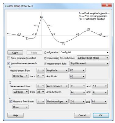
The dialog has 4 main regions: a schematic of a spike trace to use as a reference when selecting measurements, general controls, definitions of the x, y and z measurements, and the buttons to close the dialog. The dialog controls are:
