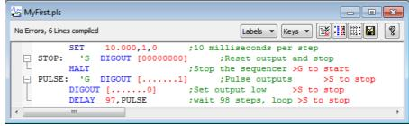
View menu Folding command and select a <u>folding style</u>), you will see that you can fold up the window text based on the keyboard codes as folding points. The Keys and Labels drop downs show a list of all the keyboard codes and labels in the file; select one to navigate to them. If you load a sequence from a read only medium or the file is marked read only, you are not allowed to change it in the editor.
