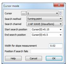
stepped along the data. Position if search fails is left blank so that if the turning point cannot be found, no measurement is taken.
