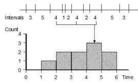
The picture illustrates how an interval histogram is formed. To make the diagram easy to understand, we have shown several events with all the intervals between them as a whole number of seconds. The interval histogram formed from these events has bins set with a width of one second.
