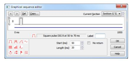
Start sampling – the sequencer will run the Initial section, which sets the starting values for all the digital and DAC outputs we have chosen to control. We did not request any other action in this section so nothing will happen until you use the G button in the sequencer control panel or select the sampling window and press the G key to start the output pulses from digital output B. You can stop the pulses with the G button in the control panel or the G key on the keyboard.
