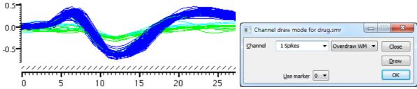
Overdraw WaveMark mode draws WaveMark data as superimposed waveforms. Channels drawn in this mode are moved to the top of the window and separated from the x axis (which does not apply to them) by a hatched bar. If this mode is used during data capture and the screen is scrolling to show the latest data, new WaveMark events are added, but old events are not erased (to stop the display flickering). Click on the x axis scrollbar thumb to force an update.
