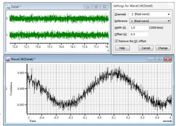
waveform moves one point to the right and the process is repeated to produce the next result. This is repeated for all the result bins. The results range between 1.0, meaning the waves are identical (except for amplitude) through 0 (uncorrelated) to -1.0, meaning identical but inverted.
