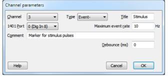
The Maximum event rate should be set to your estimate of the maximum mean event rate sustained over a few seconds. This is not the maximum instantaneous rate, which may be much higher. Spike2 uses this information to optimise buffer space allocation.
