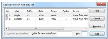
This option adds the selected waveforms to the on-line waveform output list so that they can be replayed during data acquisition. The data file must have been saved to disk. You are allowed up to 10 waveforms. As long as the list of waveforms is not full and the current waveform is less than 32 MB is size you can Add the waveform to the list. You
