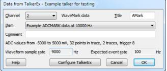
When you select a Talker in the Sampling Configuration dialog by clicking on an enabled talker name, a new dialog opens. The editable fields are:
