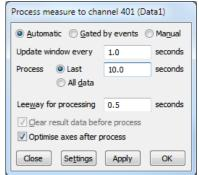
Leeway for processing is visible when processing with active cursors to an XY or time view channel. It sets the time to allow after cursor 0 for other cursors and measurements. If you set this to 2 seconds, the cursor 0 iteration is limited to 2 seconds back from the current time, allowing 2 seconds for other cursors and to take measurements. If your analysis does not generate any data, check that this value is large enough.
