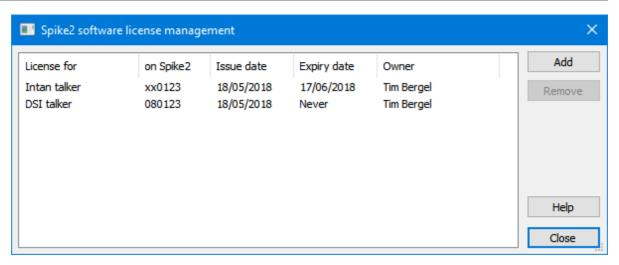
The Sample menu->Talkers->Licensing... command opens a dialog from which you can view the currently installed software licenses. Each installed license is shown on a separate line displaying: the Talker name name, owner, issue and expiry dates. Installed licenses can be selected by clicking on the relevant line of information.
