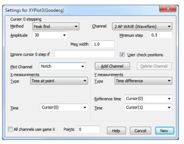
set the start and end times to XLow() and XHigh(), selected Process all data and clicked the Process button. The picture below shows the result. For each heart beat in the time range, we have a plot of the time delay from the peak to the dicrotic notch.
