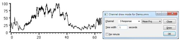
The mean frequency is calculated at each event by counting the number of events in the previous period set by Bin size. The result is measured in units of events per second unless the Per minute box is checked. The mean frequency at the current event time is given by:
