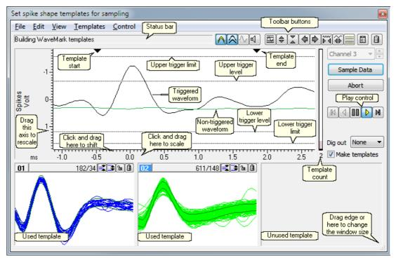
The display area shows data from the channel set by the channel control. Waveforms that meet the trigger criteria are drawn in the WaveMark 00 colour; un-triggered waveforms use the time view waveform colour.
