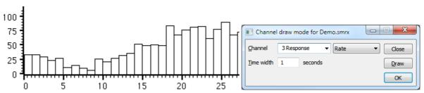
Rate mode counts how many events fall in each time period set by the Time width field, and displays the result as a histogram. The result is not divided by the bin width. This form of display is especially useful when the event rate before an operation is to be compared with the event rate afterwards.
