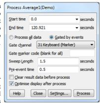
If a triggered analysis has Manual as the trigger channel, then the Start time is used as the trigger for a single sweep. In the special case of a Phase histogram with a Manual trigger, both start and end times are used to mark the beginning and end of a single cycle.
