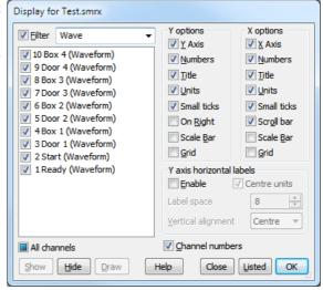
reduce the displayed channels based on matching text in the channel list. To apply a filter, type text to match into the box to the right of the Filter check box. As you type, the channel list changes to only show channels where the filter text is found in the channel identification string. The matching is case sensitive and uses <a href="ECMAScript regular expressions">ECMAScript regular expressions</a>. Clear the Filter check box to disable filtering.
