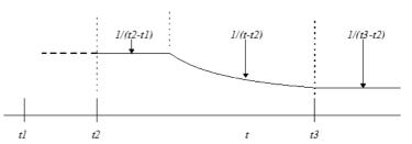
The diagram shows the result for three events at times t1, t2 and t3. From t1 to t2, the result depends on events before t1. From t2 to t2+(t2-t1), the result is set by the previous interval. From this point onwards to t3, the output reduces until at t3 it becomes 1/(t3-t2).
