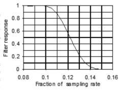
band, and reduce the filter ripple, as it widens the gap between the pass band and the stop band. If we move it back to 0.085, the attenuation in the stop band increases to 84 dB. Alternatively, we could move both edges back, keeping the width of the gap constant. This leaves the stop band attenuation more or less unchanged, but means that the start of the stop band is moved lower in frequency.
