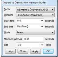
import, values that cannot be extracted from the source are set to 0. For example, when importing an event channel into a WaveMark channel, there are no marker codes or waveforms, so these are set to 0.
