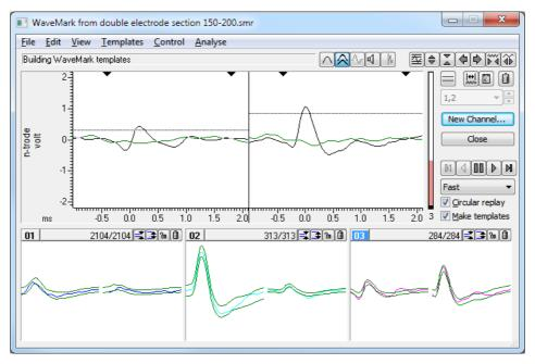
All the spike shape dialogs can handle WaveMark data with 1, 2 or 4 traces (single electrode, stereotrode and tetrode data). The documentation concentrates on the single trace case; this section explains the differences when you have multiple traces.
