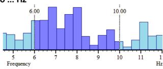
If a band starts or ends with a fraction of a bin, then that fraction of the power in the bin is included.
