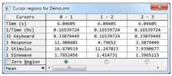
The field at the bottom left sets the measurement method; click it for a full list. Cells with no cursors or data are blank. You can interrupt long calculations in time windows with the Ctrl+Break key combination.
