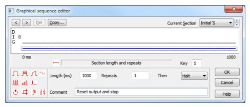
In addition to setting the initial state, we will use this section to stop our pulse output, so set the Key field to S, and set the Comment field to Reset output and stop. This comment will appear in the sequencer control panel for the S key. You can leave the Length, Repeats and Then fields at their default values (1000, 1 and Halt).
