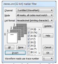
The top row of each mask represents code values 0 to 15 (hexadecimal codes 00 to 0F), the second row 16 to 31 (10 to 1F) and so on down to the bottom row, which represents values 240 to 255 (F0 to FF). If a code value is included in the filter, the corresponding element is black. When values are excluded, the element is white. The mask gives a quick indication of the state of the filter. There are three buttons that act on the entire mask:
