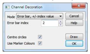
A RealMark channel holds events that each have one or more values associated with them. In a waveform display mode, Spike2 draws the one of the associated values as a wave (selected by the Draw Mode dialog <a href="Data index">Data index</a> field). The Decoration dialog allows you to use other associated values as error bars or to indicate a data range. There are currently three channel decoration modes:
