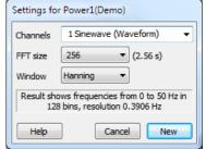
2 points in the range 16 to 262144. You set the FFT block size from a drop down list. The result window ends up with half as many bins as the FFT block size. When you use the Process command, the selected area must hold at least as many points as the block size, otherwise no analysis is done.
