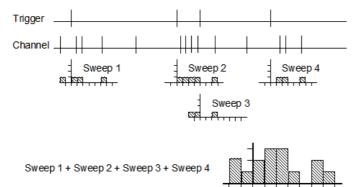
This command performs event cross-correlations and event auto-correlations between a trigger channel and one or more other event channels. A cross-correlation produces a measure of the likelihood of an event on one channel occurring at a time before or after an event on another channel. The result can be displayed as a spike rate or as a count.
