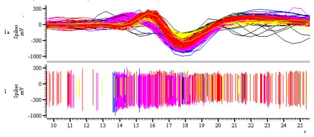
In Overdraw WM mode, the full width of the window is used for each spike. There is a grey bar between the overdraw area and the rest of the window to show that the x axis does not apply. When the window scrolls, new spikes are added to the overdraw area, but old spikes are not removed as this would force the entire window to redraw, which could take a long time. If you want to force the overdraw area to redraw, click or drag the thumb in the scroll bar at the bottom of the window.
