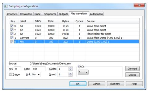
Wave identifier. A character or two hexadecimal digits in <u>marker code format</u>; you may not repeat a code or use 00. It is added to the <u>Keyboard marker channel</u> on a <u>Play wave toolbar</u> button click.
