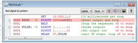
marked by changing the background colour and an explanatory message is shown at the top of the screen. Any edit to the sequence will remove the background colour change. The compiler stops at the first error it finds. If the compiler completes without error is display the number of sequencer lines (instructions) that were compiled. The compiler always adds a HALT instruction to the end of the sequence, so the count will be one more than the number of listed lines.
