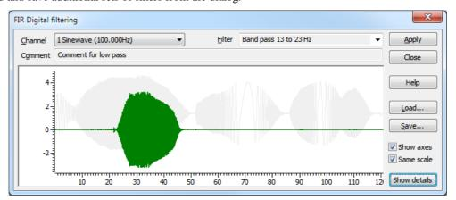
The dialog shows the original waveform in grey, and a filtered version in the colour you have set for waveform data in a time view. Whenever you change the filter, the display updates to show the effect of the change.
