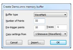
Channels created with this command are not permanent. The data is kept in memory and is lost when the file is closed. If you need to make the data permanent, you must write it to a permanent channel with the Write to Channel option.
