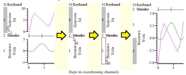
Channels 1 and 3 now share the same space with the channel numbers stacked up next to the Y axis. The visible Y axis is for the top channel number in the stack. You can promote another channel in the stack to the top by double-clicking the channel number. The channels retain their own y axes and scaling. You can remove a channel by dragging the channel number to a new position.
