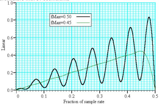
If you must span the full range, use an even number of coefficients. The graph below shows the improvement you get with an even number of coefficients. The ripple for the 0.45 case is about the same with 10 coefficients as for 31.
