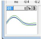
In small mode, the four rectangles at the top of the template hold, from left to right, the code associated with the template (01), the number of spikes in the template (8), a button that indicates the locked state of the template and a button that can be used to delete the template. The vertical size of the displayed template is set by the vertical scale of the data display area.
