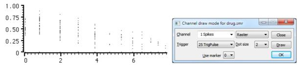
Raster mode shows the event positions relative to trigger times. Each trigger event defines time 0 in the y direction for the sweep. The Y Range dialog sets the time range to display in the y direction; negative times show pre-trigger events. For each trigger, events are drawn no further back in time than the previous trigger and no further forward in time than the next.
