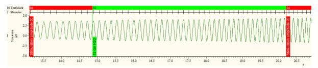
The picture shows an example of the use of vertical markers with a TextMark channel being drawn in both state mode and as a vertical marker. Vertical markers are often used in place of vertical cursors where you need a marker that cannot be moved by the user. If you use a memory channel as the vertical marker channel, you can edit the position by adding and removing items in the memory channel.
