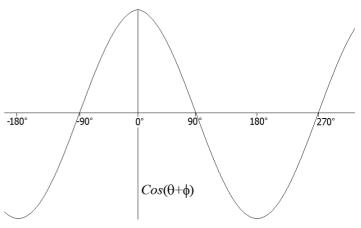
By adjusting  $\phi$  you control the output cosine phase where  $\theta$  passes through zero. Unless you set the value (PHASE), it is zero and the zero crossing occurs at the peak of the sinusoid. To have the output rising through 0, set the phase to -90.
