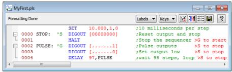
panel. You can remove step numbers with the Format button. Lines that get a number are part of the sequence run by the 1401. The <u>SET</u> line tells the sequencer how fast to run, in this case 10 milliseconds per step, and is not part of the sequence run by the 1401. A SET or <u>SCLK</u> directive is usually the first line in the sequence.
