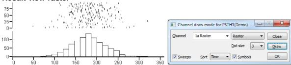
If a result view channel has associated raster data, there are two more drawing modes: Raster and Raster lines. Raster mode shows each event as a dot, Raster lines mode shows each event as a short vertical line. The Dot size field controls the dot size and vertical line length. In Raster lines mode you can check the Centre line box for a horizontal line through each sweep.
