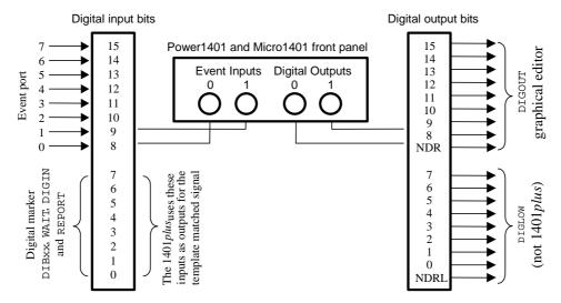
The digital input and output ports are 25-way connectors. The data and ground pins are the same on both. See your 1401 Owners Manual for full details of all pins.
