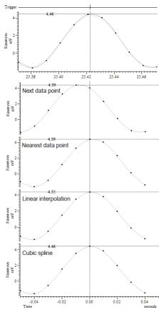
If your data contains transients with frequency content above half the sampling rate, cubic interpolation will become inaccurate and the best you can do is choose the Nearest data point method. The Next data point method is provided for backwards compatibility with older versions of Spike2.
