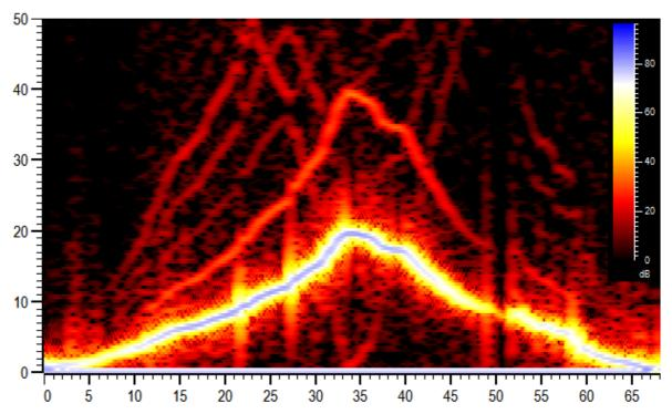
Sonogram mode shows how the frequency content of a waveform channel changes with time. The y axis units are Hz (frequency) and useful results are available for the frequency range 0 to one half of the sampling rate for the waveform channel. You can control the <u>colour scale</u> used for the sonogram and display a key to indicate how the colours map to intensity.
