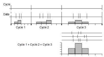
A phase histogram is used to show how events are distributed with respect to a cyclical process that may vary in cycle time. One event channel marks the start and end of cycles. The end of one cycle is the start of the next. Events on another channel are placed in bins depending upon their position within each cycle.
