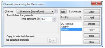
list. Delete removes the selected process. When recording is enabled, Apply copies changed argument values to the process and records the script to make the change, otherwise changes are applied immediately.
