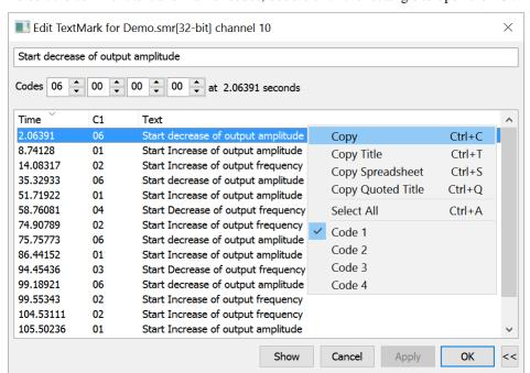
The <u>marker codes</u> display in the format set for the source channel (<u>Hex only or using printing characters</u>). Regardless of the channel format, you can always set the code in either format (two hexadecimal digits or one printing character).
