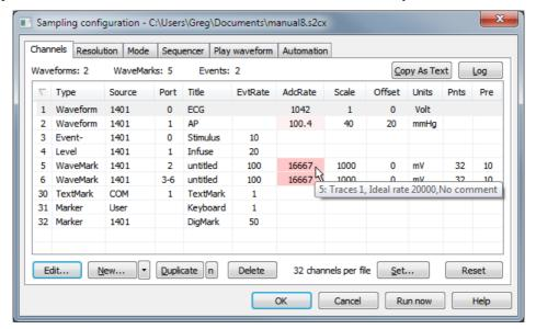
The top line displays counts of Waveform channels, ports used for WaveMark channels and event channels plus controls to copy the configuration as text to the clipboard or to the Log window. You edit the channel settings by double-clicking on a channel, or by selecting a channel with the mouse or keyboard and clicking the Edit button. The Reset button deletes all editable channels and sets a standard sampling state.
