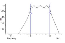
circles vertically or with the Ripple field to the right of the displayed frequency response. You will likely select this type of filter when having no signal in the stop band is more important to you than the flatness of the pass band and you do not care about preserving the signal shape.
