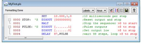
allowed) and can pinpoint the line where your sequence is not behaving as you expect. When your sequence is running, the <u>sequencer control panel</u> displays the current sequencer step. A number at the start of a sequencer line is completely ignored when sequences are compiled, so you need not worry about editing a sequence that has step numbers. Just format the sequence to clean up the changes.
