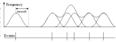
The diagram shows the result of using the built-in raised cosine waveform. The area under the curve for each spike is 1. You would normally use a smoothing period that covered several events to obtain a smooth output.
