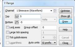
waveform channels and from 0 to the estimated event rate for event channels drawn with a frequency axis. Both these buttons close the dialog. You can optimise without opening the dialog with the keyboard short-cut Ctrl+Q and by right-clicking on a channel and selecting the Optimise option from the context menu. In logarithmic mode, values of zero or less cannot be displayed.
