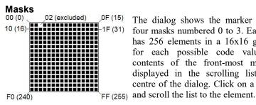
The dialog shows the marker filter as four masks numbered 0 to 3. Each mask has 256 elements in a 16x16 grid, one for each possible code value. The contents of the front-most mask are displayed in the scrolling list in the
