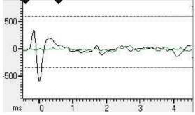
The two black triangles mark the start and end of the region of the spike that is passed to the template matching system. Click on a triangle and drag to change the region. When you drag the markers, vertical cursors drop down to identify the selected area.
