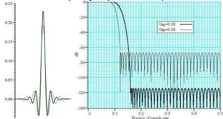
The frequency response is shown in dB, which is a logarithmic scale. A ratio r is represented by 20  $\log 10(r)$  dB. A change of 20 dB is a factor of 10 in amplitude, 6 dB is approximately a factor of 2 in amplitude. The graph shows that a frequency in the stop band is attenuated by over 110 dB (a factor of 300,000 in amplitude with respect to the signal before it was filtered).
