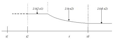
The diagram shows the result for three events at times t1, t2 and t3. From t1 to t2, the result depends on events before t1. From t2 to t2+(t2-t1), the result is set by the previous interval. From this point onwards to t3, the output reduces until at t3 it becomes 1/(t3-t2).
