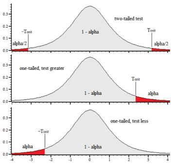
your alpha value is 0.01 and this is the value to test for. Due to the symmetry of the distribution, to test that "this mean is less than that mean" you need a negative t value; the probability to test for is the same as for a positive t value. A one-tail test should be used with caution.
