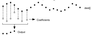
This diagram shows how the FIR filter works. Open circles represent filter coefficients, solid circles are the input and output waveforms. Each output point is generated by multiplying the waveform by the coefficients and summing the result. The coefficients are then moved one step to the right and the process repeats.
