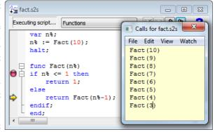
generate a factorial (but see <u>LnGamma()</u> and <u>BinomialC()</u> for large factorials). Excessive call stack use is trapped and will stop a runaway recursive script (unless it runs out of memory before hitting the stack limit).
