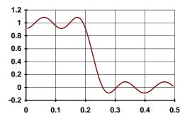
This is illustrated by these two graphs. They show the linear frequency response of two low pass filters, both designed with 18 coefficients (we have used so few coefficients so the ripple is obvious). Both have a pass band of 0 to 0.2, but the first has a gap between the pass band and the stop band of 0.1 and the second has a gap of 0.05. We have also given equal weighting to both the pass and the stop bands, so you can see that the ripple around the desired value is the same for each band.
