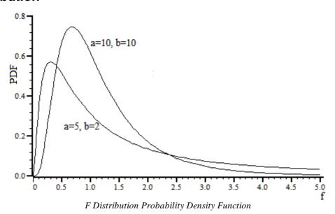
The <u>F Distribution</u> probability density functions shows the likelihood of particular values of the F statistic occurring. The F statistic calculation depends on the situation; in a simple case it is the ratio of two variances. The F distribution can be calculated and displayed by the script code:
