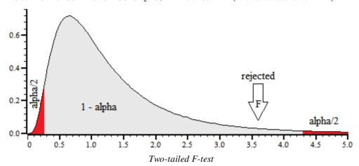
Given this result, for a two-tailed test the hypothesis that the standard deviations are different is rejected at the 5% level as the F statistic does not fall outside the range 0.259411 to 4.29513. The probability value returned (that the result occurred by chance) is for comparison with alpha for a one-tailed test; for a two-tailed test compare it with alpha/2 or double it for comparison with alpha .
