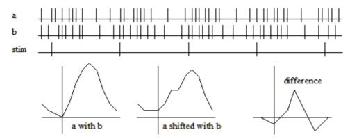
If the stimulus channel holds events at some constant interval int, by shifting all events on one of the two channels by int, the only correlation between the two channels left is the correlation due to the stimulus. Thus by forming the difference between the unshifted correlation and the shifted correlation, you can obtain the correlation between a and b with the effect of the stimulus removed.
