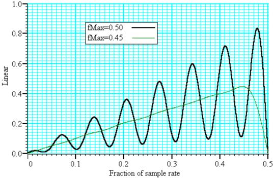
If you must span the full range, use an even number of coefficients. The graph below shows the improvement you get with an even number of coefficients. The ripple for the 0.45 case is about the same with 10 coefficients as for 31.
