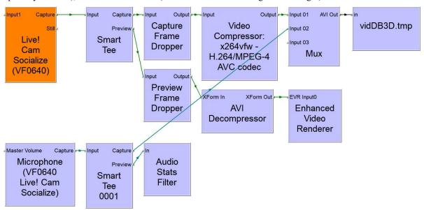
The arrows show the direction of data flow between the filter *Pins* (a pin is a possible connection point of a filter). The various filters that can appear in the graph are:
