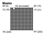
The dialog shows the marker filter as four masks numbered 0 to 3. Each mask has 256 elements in a 16x16 grid, one for each possible code value. The contents of the front-most mask are displayed in the scrolling list in the
