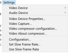
The final section holds links to the Configuration menu, where you choose how (or if) the video and audio streams are compressed and the codecs used. It also holds the Slow Frame Rate controls (used to reduce the quantity of video information during uninteresting data capture).
