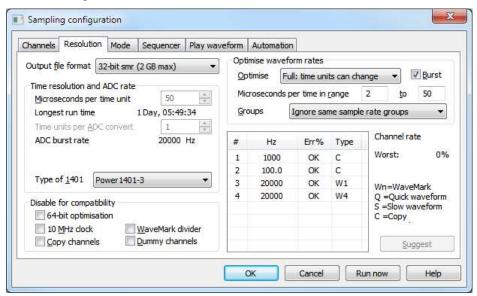
In this example, setting burst mode allows us to run for more than 1 day when sampling to a 32-bit file (1 Waveform at 1 kHz, one at 100 Hz, a WaveMark channel with 1 trace at 20 kHz and another with 4 traces). Without burst mode, the time resolution has to be 10 microseconds, which limits the run time to just under 6 hours. Of course, if you target a 64-bit file, you can run at 1 microsecond resolution with no practical time limit.
