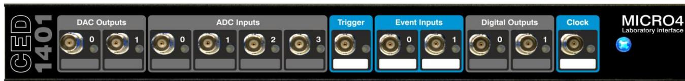
**Clocks** The Micro4 has four clocks. The event clock times and counts external pulses; the general-purpose clock generates timing pulses; the ADC clock controls waveform input sampling rate; the DAC clock controls waveform update rate, but DACs can also be updated by the ADC and general-purpose clocks. These clocks are managed automatically by the application.
