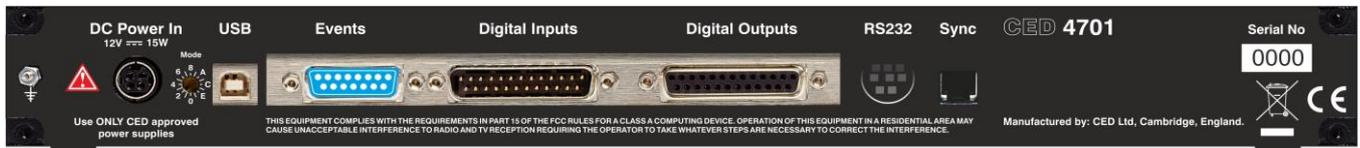
**Event inputs** The rear-panel Events D-socket provides more clock-related inputs, the Clock E series and Clock F. These inputs allow 1401 programmers close control of the clocks. Details are given in the *1401 family programming manual*, and the *Micro1401-4 technical manual*. The front-panel BNCs Event 0 and Event 1 are often routed by software to the Clock E0 and E1 inputs.
