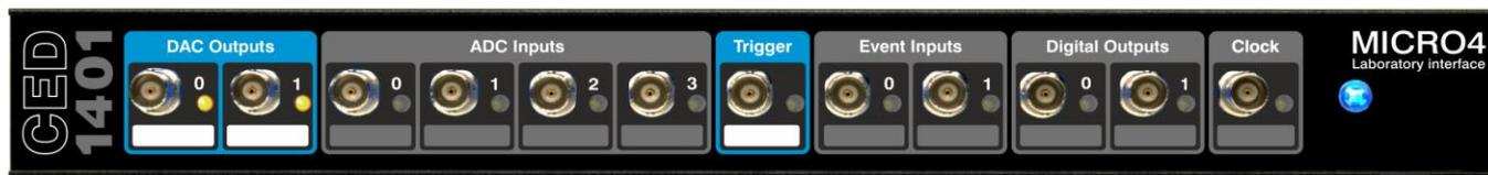
**Waveform output** There are two, optionally four, waveform output channels on the Micro4. The standard pair, DACs 0 & 1, outputs through BNC connectors on the front panel labelled DAC Outputs. The optional DACs 2 & 3 may be routed to BNC connectors on the rear panel, or come out through an expansion top-box.
