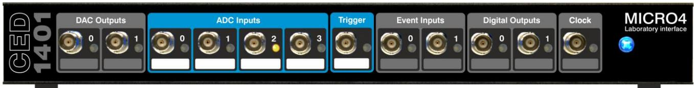
**Waveform input** Waveform input channels are buffered through unity-gain amplifiers. Signals are then steered into the ADC (analogue to digital converter) via a multiplexer. The input sample-and-hold is part of the ADC chip. The ADC converts an input voltage to a 16-bit digital value in approximately 1  $\mu$ s.
