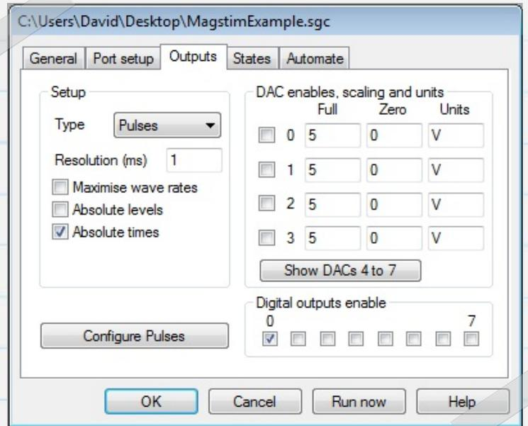
If using a BiStim<sup>2</sup> in IBT mode you will need to enable two digital outputs, one to trigger each of the units of the BiStim<sup>2</sup>
