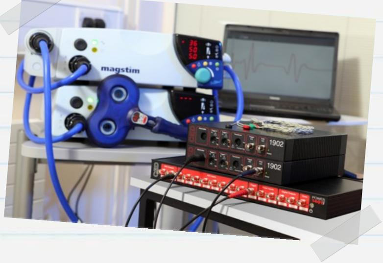
Signal is a sweep-based data capture and analysis software package. It provides direct control of Magstim stimulator parameters during sampling, including adjustment of stimulus intensity and trigger timing. This guide is intended to help you setup a TMS system for evoked potential recording using Signal, a 1401 interface, a 1902 amplifier and a Magstim stimulator.
