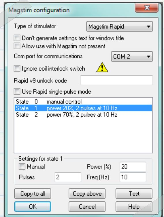
The **Ignore coil interlock switch** option disables the switch on the Magstim coil handle so that the device will fire in response to triggers without the button being depressed. Magstim do not recommend bypassing the switch as this is a safety feature and should not be used unless absolutely necessary. Rapid devices with the latest version 9 firmware require an unlock code, as an additional safety precaution. The unlock code for these devices can be obtained by contacting Magstim.
