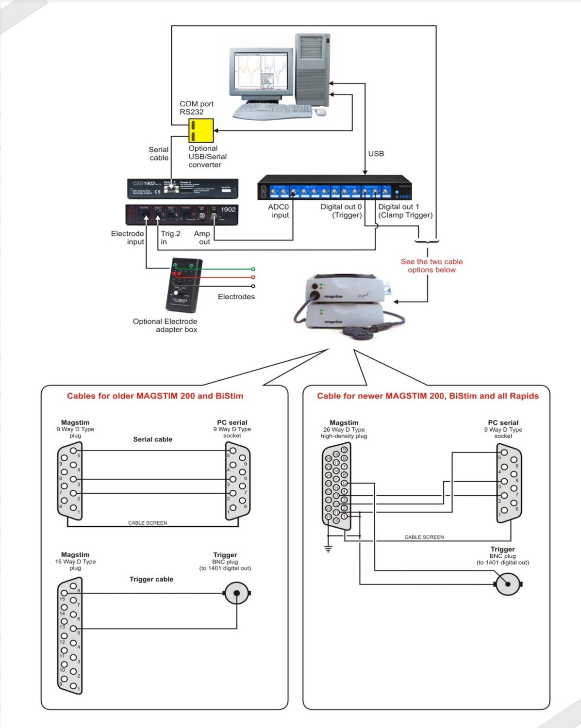
In the diagram above the CED 1902 is fitted with an input clamp option, which can be used to suppress the artefact that occurs after stimulation. This is generally only required with very fast responses (i.e. 2–10ms after stimulation), or if recordings are taken close to the site of stimulation. The input clamp is triggered with an input to the Trigger 2 port on the 1902 as shown. See [1902 amplifier setup](#) for further details.
