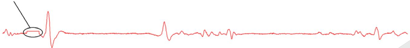
Stimulus artefacts can often saturate the input of an amplifier, causing a period of 'lost' recording while the amplifier input returns to a normal level. This can cause problems if the response is very fast or is being recorded from close to the site of stimulation. The diagram above shows a fast MEP response from the electrode (Fig. A) that is missed due to the amplifier saturation caused by the stimulus artefact (Fig. B).
