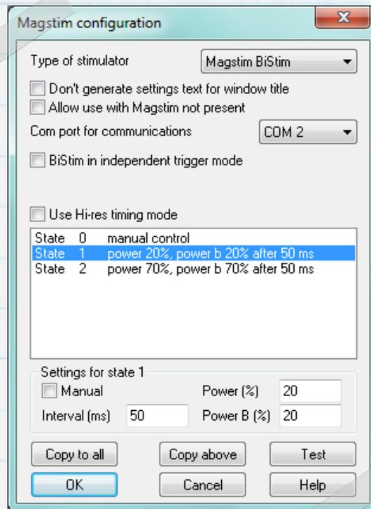
Setting an interval of Zero switches the BiStim into simultaneous pulse mode. In this mode both stimulators must use the same power level, which is taken as being the main Power setting in the configuration, with the power b setting ignored.
