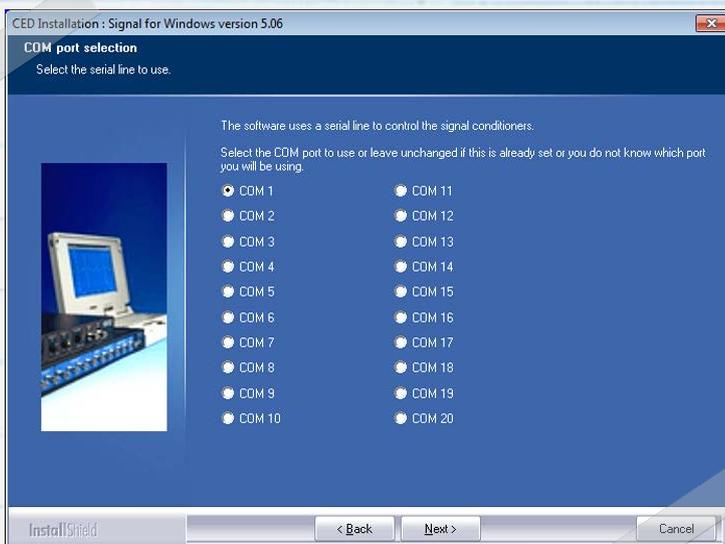
The CED 1902 amplifier is controlled via a COM port (RS232). Many desktop PC's will have at least one COM port available (usually COM1). For laptops and PCs without an available COM port, a [USB to serial adaptor](#) can be used instead. This should be plugged in to an available USB port before continuing.
