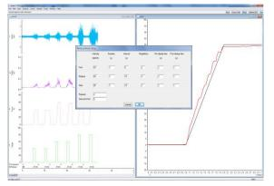
Force-time target following experiment. Script generated target template with overlaid subject response. Target recorded in data file with associated EMG
